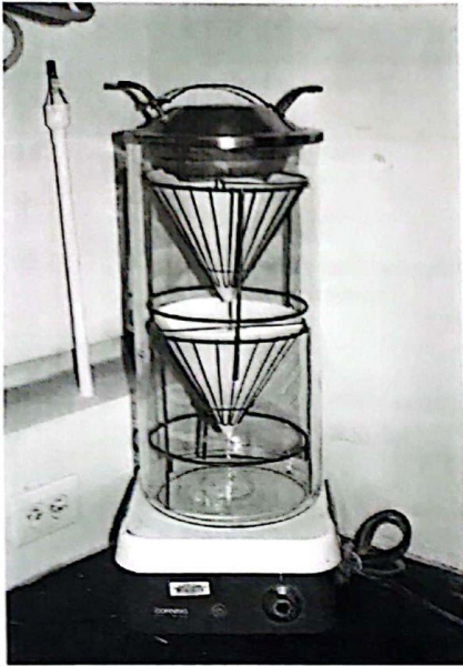
Figure 2 —Extraction Apparatus (Method B)
