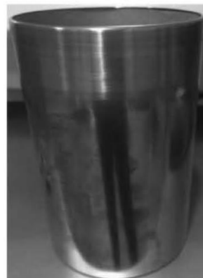
FIG. 3 Centrifuge Cup with Inlay Paper
